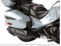
SELF-LEVELING AIR SUSPENSION Rear air shocks automatically adjust to passenger and cargo weight to ensure comfort is never compromised.
